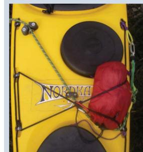
A kayak mounted towline reduces the strain on the paddler, it is usually fitted by means of a fairlead (eye) and a jamming cleat fixed on the deck behind the cockpit. When fixing the eye and cleat make sure a strong backing plate and large washers are used to spread the load. Positioning the tow in the middle of the kayak allows for greater manoeuvrability (a harbour tug has the anchor dead centre).
